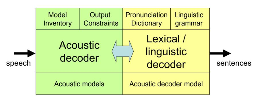
Different modules are used for the acoustic modelling and the lexical / linguistic modelling
